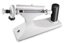
Cuvette in measuring chamber
