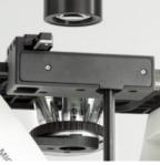
Coaxial control knobs for x/y can be fitted either left or right
